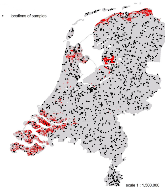
Figure 1. Locations of the national stratified soil survey sampling (Finke et al., 2001). The red area is an example of the location of one of the 95 strata (calcareous silty clay soils with a MHW between 0.4 and 0.8 m) that is distinguished in the national stratified soil survey.
