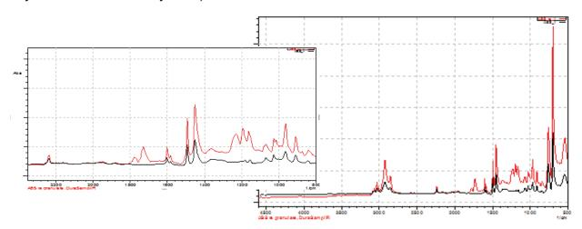
FTIR Spectra of virgin and post consumer waste. Additional peaks appear, especially over the region 2000- 1000 cm-1. The material could be contaminated with polycarbonate or a brominated flame-retardant.
