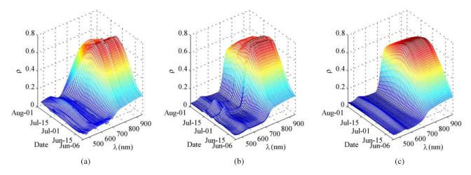
Fig. 2. STRS of experimental plot one created by (a) direct spectral-temporal interpolation; (b) first imputing the Formosat-2 spectra and then performing a temporal spline interpolation; and (c) proposed Bayesian approach including sensor uncertainties.
