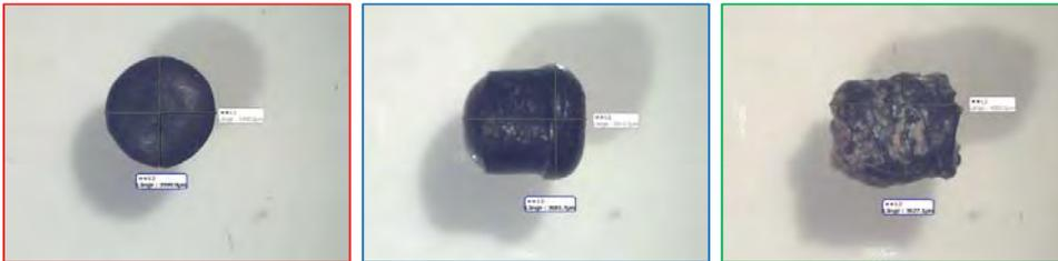
Beached pellets are, especially on the surface, exposed to UV-radiation, heat and sand (grinding).
