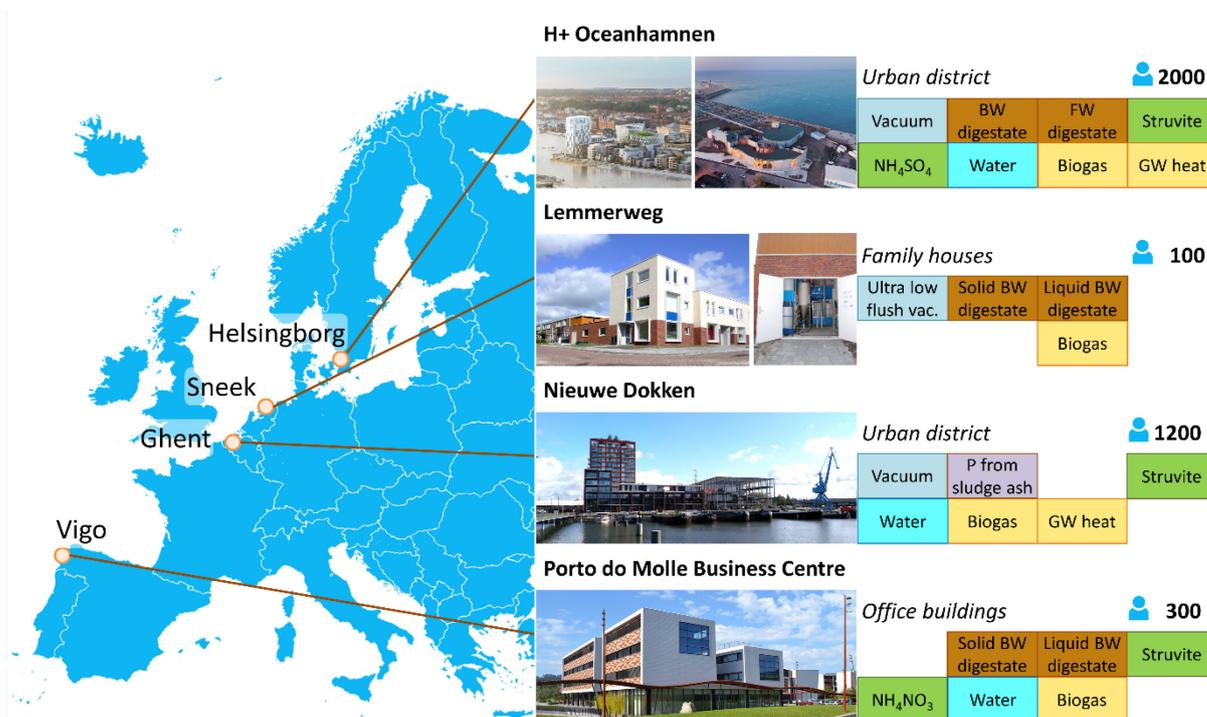
Figure 2: Overview of the four demonstration sites of the Horizon 2020 project Run4Life and the resources recovered at each site ([www.run4life-project.eu](http://www.run4life-project.eu)).
