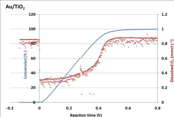
The top picture shows the conversion of a carbohydrate over time (blue line, left axis), and the dissolved oxygen concentration during reaction (red line, right axis). In this case the oxidation is performed using a low surface area catalyst support (Au/TiO<sub>2</sub>). As can be seen from the red line, the oxygen concentration stays low during reaction, thereby limiting the conversion rate.
