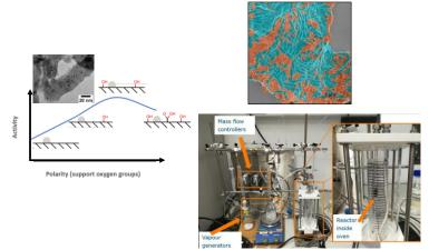
Some examples: Influence of surface oxygen groups on the activity of Pt/CNF for electrochemical glucose oxidation (left). SEM visualization of starch (RS3, orange) by rod shaped bacteria (blue) (top right). Rebuild CO2 capture setup (bottom right)
