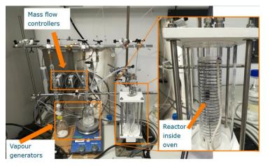
Fig 1: Picture of CO<sub>2</sub> capture setup
