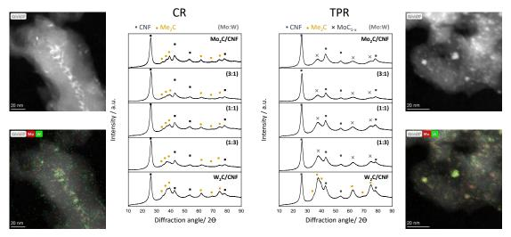
Figure 2. TEM-EDX and XRD diffractogram of carbide catalyst synthesis via the temperature-programmed reduction under 20%  $CH_4/H_2$  (TPR, left) and via a carbothermal reduction in  $N_2$  (CR, right)
