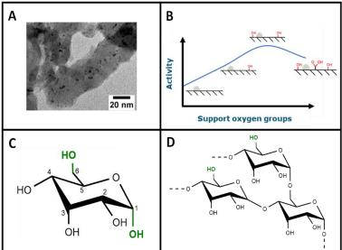
Figure 3. A) Self-synthesized nano-sized Pt particles decorated on carbon nanofibers. B) The relation between support oxygen groups on CNF on the electrocatalytic activity of Pt towards glucose oxidation. C) Where it was found that Pt can be used for the oxidation of the  $C_1$  and  $C_6$  groups of glucose. D) shows the aim for next year, where we aim to oxidize starch at the  $C_6$  group.
