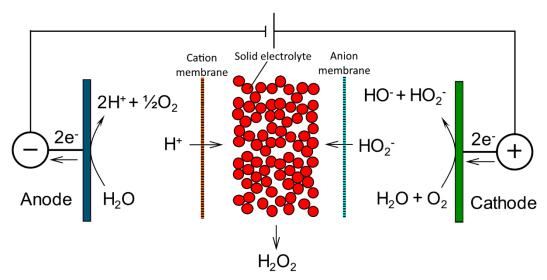
Figure 4: Cell design for electrochemical hydrogen peroxide production in HYPER project
