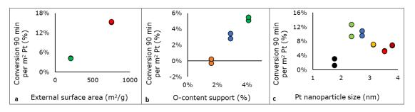
Figure 1: Oxidation of starch (%) with duplicate experiments over different types of supported solid catalysts. Catalytic activity increases with increasing surface area (a) and polarity (i.e., amount of O-groups, b) of the carbon support. Small nanoparticle sizes of Pt exhibit low activity due to deactivation, and large nanoparticles have low activity due to the low surface area of Pt. Nanoparticles of 2-3 nm are shown to be the most active (c).
