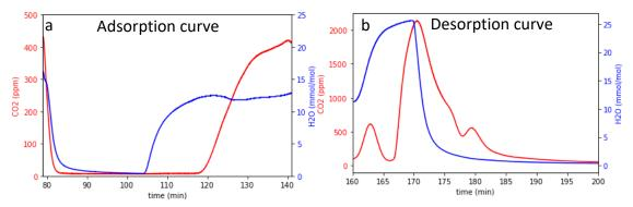
Fig 2: Adsorption and desorption curves (gas concentrations at reactor outlet). CO2 concentration in red H2O concertration in blue. (a) concentration remains 0 while sorbent removes CO2 from air, increases again when sorbent has reached capacity. (b) Sorbent heated to 200C with 10C/min under nitrogen higher concentrations mean more gas is desorbed from the sorbent, until it reaches 0 and everything is desorbed
