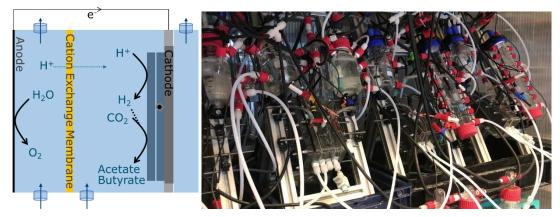
Figure 5. Schematic (left) and actual (right) setup of bioelectrochemical chain elongation systems.
