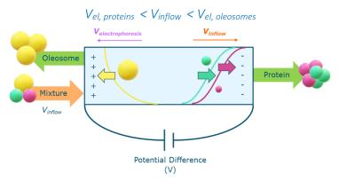
Figure 1: Schematic representation of the continuous electrophoretic extraction process.
