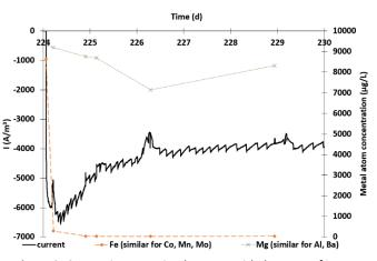
**Figure 2.** Current increase simultaneous with decrease of iron, cobalt, manganese and molybdenum from the liquid. The decrease from the liquid indicates they were deposited on the cathode.<sup>[1]</sup>
