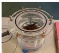
Figure 4 Fiber optic microsensor in ray egg
