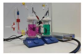
Figure 1. H-cell used for preparative electrolysis.
