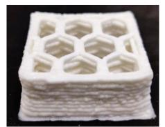
Figure 5: 3D printed honeycomb structure of pea protein stabilized jammed emulsion
