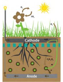
Concept of a plant microbial fuel cell.
