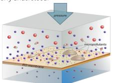
Fig 1 Schematic illustration of the processes at the highpressure side of a membrane that retains micropollutants from surface water For instance, because of the general hydrophobic nature of micropollutants, they may condense into nano-droplets on the membrane surface (Fig 1) and affect the transport and overall process. In this project, this phenomenon is explicitly considered together with intramolecular and particle-surface interactions.
