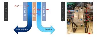
For many applications, the exact ionic composition is crucial. For example, the horticulture wastewater can be rich with nutrients (e.g.,  $Ca^{2+}$ ,  $NH_4^+$ ), however, the high sodium concentrations limit its reuse. In this case, a selective removal of Na<sup>+</sup> is required. We will consider the effluent requirements of the desalinated water (diluate) as well as the environmental compatibility of the concentrate stream. Key objectives:
