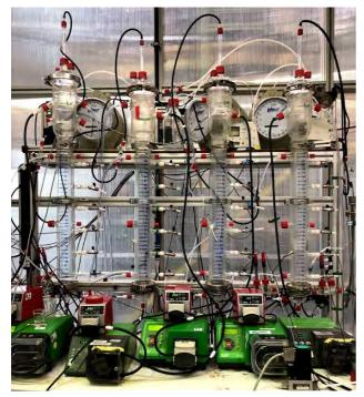
Figure 1 Lab-scale UASB reactors
