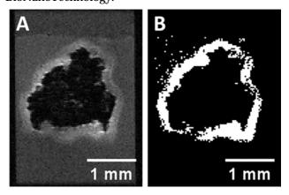
Figure 1. (Above) An example of biofilm on electrode material measured with MRI (A), and the image after threshold analysis (B). Taken from Caizán-Juanarena et al. (2019).
