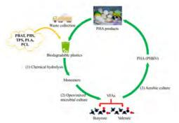
Fig.1 Biodegradable plastics closed loop recycling
