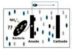
Figure 2 Concept of an anaerobic ammonium oxidation bioelectrochemical system integrating with electricity recovery.
