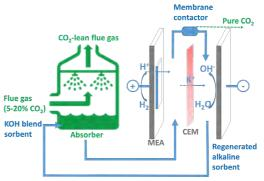
**Fig. 2**. Schematic illustration of the CO<sub>2</sub> capture process based on absorption in alkaline (KOH) blend and electrochemical regeneration.
