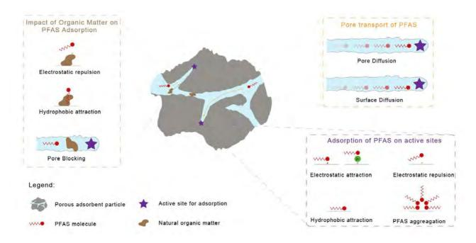
Figure 1. Mechanistic interactions between PFAS and adsorption material that will be studied
