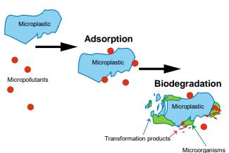
Fig. 1: Experimental approach to investigate the adsorption of organic micropollutants to microplastics and their biodegradation by microbial communities
