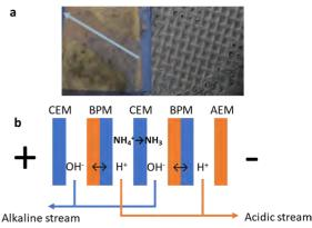
Figure 1. (left) Inorganic scaling of CEM in ES ammonia recovery. MEA: membrane electrode assembly, CEM: cation exchange membrane, ED: electrodialysis, LLMC: liquid-liquid membrane contactor. Figure 2 (above) a. Inorganic scaling in CEM and spacers of ES. The arrow shows the direction of the flow. b. ES with possible production of acidic and alkaline streams. The possible use of these streams still needs investigation. AEM: anion exchange membrane, BPM: bipolar membrane.
