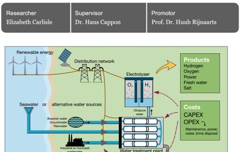
water treatment plants. We also plan to model various water treatment technologies. Several different options for water treatment can be used, based on the quality of the source water: reverse osmosis, forward osmosis, membrane distillation, or electrodialysis, for example. In addition, the future energy and water availability are uncertain, necessitating the use of stochastic programming or similar methods.
