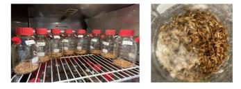
Batch-mode BWO reactor & woody substrate colonized by fungi.
