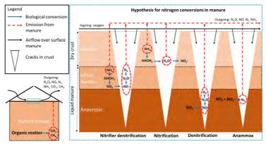
Figure 2. hypothesis of the nitrogen conversion pathways taking place in anaerobically stored manure as well as in the crust layer during storage.
