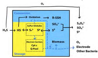
Figure 1 A simplified overview of the postulated mechanics of sulfide conversion and storage yellow field), and electron transfer (blue striped lines).
