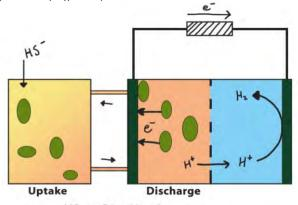
HS  $\rightarrow$  S0 + H<sup>+</sup> + 2e Figure 2 A simplified sketch of a sulfide removal SOB fuel cell.
