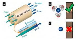
Figure 2. A) Reverse-osmosis and nanofiltration are pressuredriven separation technologies. B) Charged ions, in this case boron (B-), are successfully rejected by the membrane, while C) uncharged solutes can pass.
