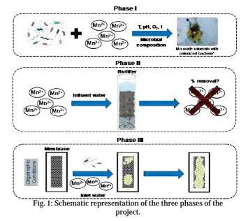
The project consists of three phases (Fig. 1): (I) exploring the dynamics/kinetics of biogenic Mn oxidation by mixed microbial consortia, (II) studying Mn removal in diverse lab-scale biofilters, and (III) understanding the fouling dynamics related to Mn in oligotrophic conditions. The goals are:
