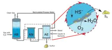
Fig. 1 - Schematic of the current biodesulfurization process and the shuttling capacity the occurs between the anaerobic (AN) and the aerobic (AE) reactors.
