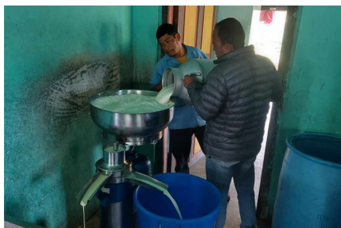
Figure 4: Cream separating at Milk Processing Unit (MPU).
