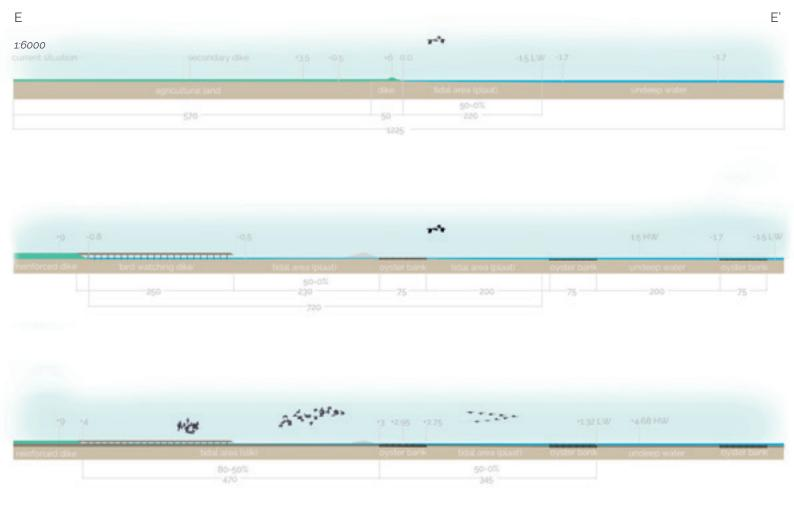
Fig. 70. A - Transition from the existing situation (top), the intervention (middle), and the 'final' situation (down). By silt suppletions, the tidal area silts up heigher and oyster banks grow with SLR. Dimensions in m, heights in relation to NAP. HW: high water level, LW: low water level.
