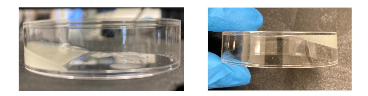
Figure 3. UV-cured microalgae-based resin.
