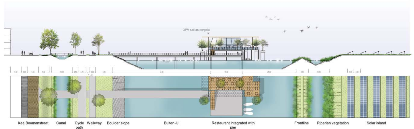
A new restaurant on piles refers to Amsterdam's peat soil conditions and provides an elevated view of the solar island, lake Buiten-IJ and surroundings. People can access the pier any time, subsequently deciding if they want to experience a more elevated view on the restaurant's terrace during opening hours.
