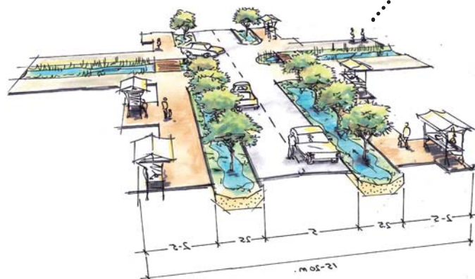
Improved roads separated by bioswales
