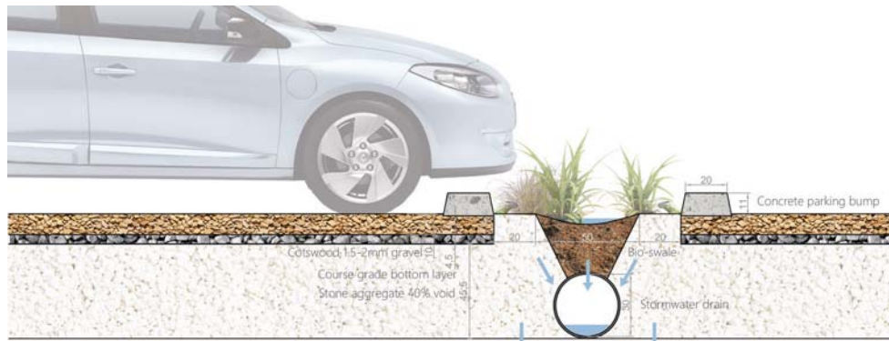
Permeable parking lots could create a strip of urban flood plains along the entire Shore.
