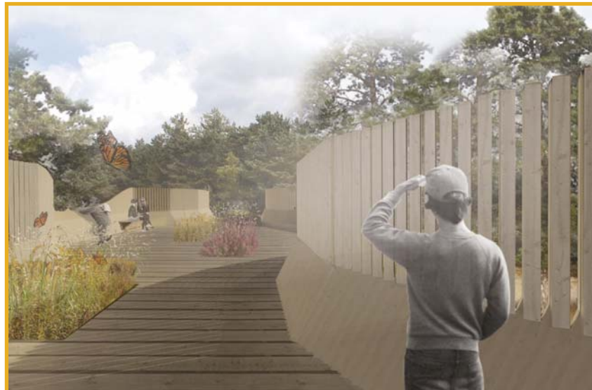
▲ Pedestrian bridge over A12 intervention The aim is to provide a solution for both a broader view on nature and other multi-sensory stimuli, and for hiding the negative phenomenon of the highway. The proposed solution is the concept of the semi-transparent fencing - from certain angles a transparent fence, from others a solid wall blocking the view - to create a visual barrier towards the highway but allowing a broad view on the natural environment. This alone does not eliminate the noise, however a rich experience can reduce the negative effect of the noise on the experience.
