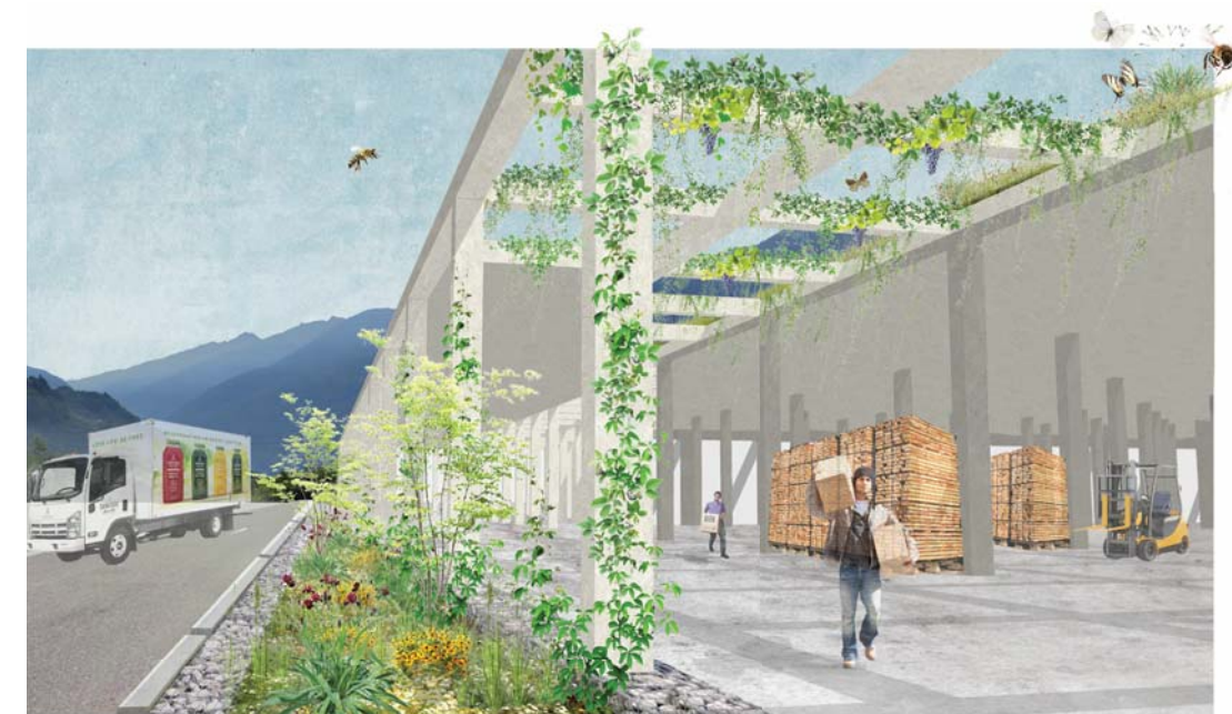
The structure works partly as a green roof to hide but also to catch water. Partly it works as a pergola.
