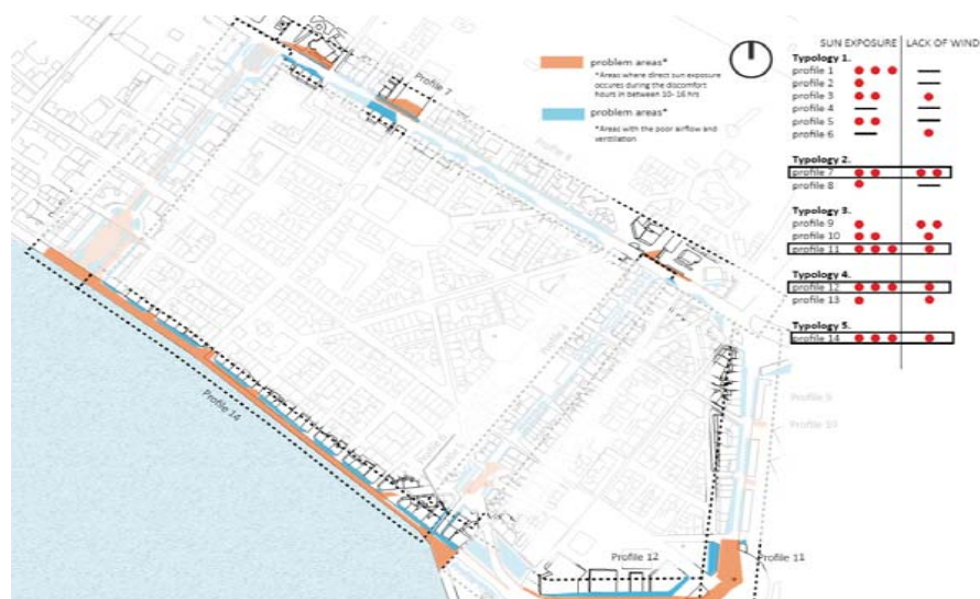
Overlap of the shadow and wind analysis is resulted in the four most problematic profiles, that serve as a basis for the test-beds.
