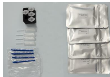
Figure1. LFD Kit content; Left (top to bottom) reaction tubes with buffer and support, mini pipettes (4x), pestles (4x), Right pouches with cassettes strips (4x).
