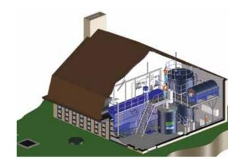
Figure 3: 3D-representation of Novel Sanitation in Sneek, Noorderhoek (left panel). The facility treating source separated streams and producing clean water, biogas, electricity, and phosphorous solids, is placed in one central building (right panel) to which the 232 houses are connected.
