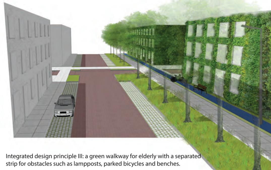
Integrated design principle III: a green walkway for elderly with a separated strip for obstacles such as lampposts, parked bicycles and benches.
