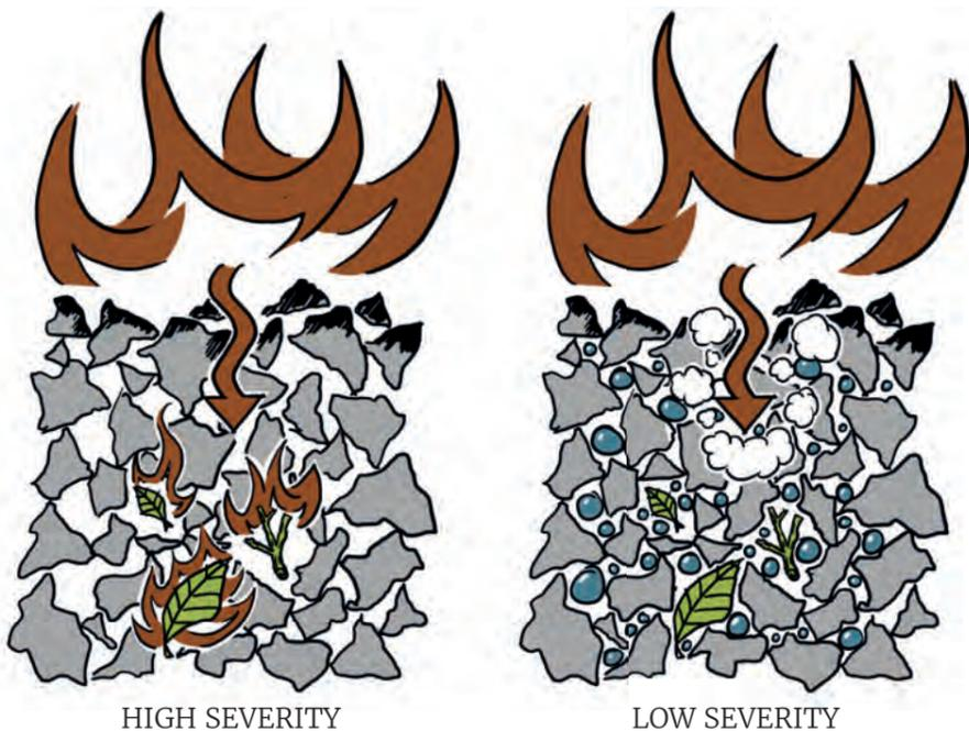
The difference between a high severity fire (left) -where much organic material is burnt due to low moisture levels- and a low severity fire (right) where less organic matter is burnt as more moisture is present in the landscape and soil.
