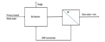
Figure 1 The proposed process, a combination of nanofiltration and biological treatment
