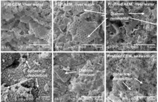
Fig 2. Fouled membranes with river and sea water, different types of AEMs and CEMs. Adapted from [2]
