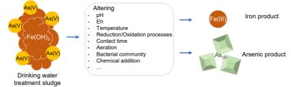
Figure 1. Proposed scheme for iron recovery and arsenic isolation
