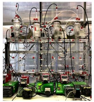
Figure 1 Lab-scale UASB reactors
