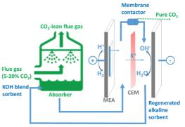
**Fig. 2**. Schematic illustration of the CO<sub>2</sub> capture process based on absorption in alkaline (KOH) blend and electrochemical regeneration.
