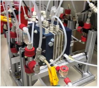
**Figure 2:** Microbial electrolysis cell removing ammonium from wastewater.
