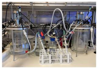
Continuous operation of bioreactors.
