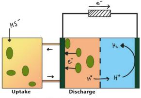
HS<sup>•</sup>  $\rightarrow$  S0 + H<sup>+</sup> + 2e<sup>•</sup> Figure 2 A simplified sketch of a sulfide removal SOB fuel cell.
