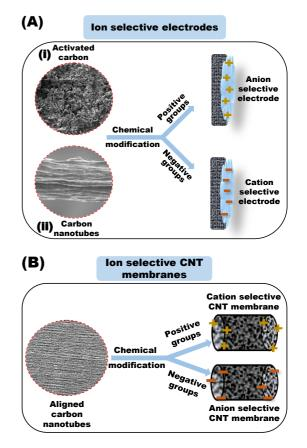
Fig.1: (A) Preparation of ion selective carbon electrodes from (i) activated carbon (AC) and (ii) carbon nanotubes (CNTs). (B) Chemical modification of aligned carbon nanotubes (CNTs) to prepare an ion-selective membrane.
