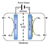
Methane-producing BES:  $CO_2$  is converted to methane by mixed culture microorganisms at the cathode side while at the anode water oxidation provides the protons and electrons necessary for reduction of  $CO_2$ .
