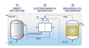
to keep methanogens at optimal metabolic activity. Finally, to reach efficient methane production, individual mass and energy flow need to be optimized in terms of energy requirements (kJ/mol CO2), and product yield (mol CH4/m3 air).
