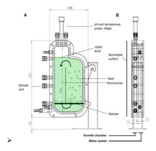
Fig. 1 Design of the lab-scale PBR
