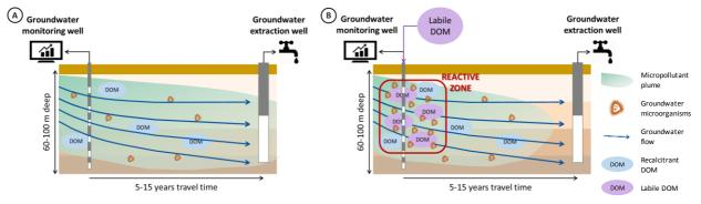
Micropollutant attenuation in groundwater: A - Natural attenuation; B - DOM amended attenuation
