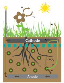
Concept of a plant microbial fuel cell.
