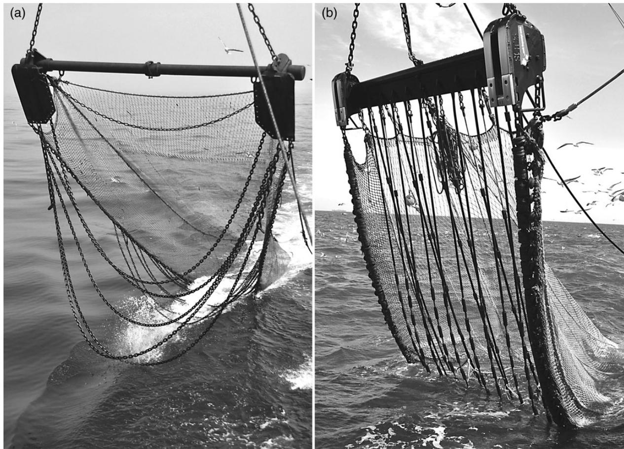
**Figure 3.** Commercial tickler-chain beam trawl (a) and pulse trawl (b) used in the experiments.
