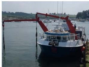
b) Vessel with a « scoubidou », used to harvest Laminaria digitata on the coasts of Brittany (France) © Maguire
