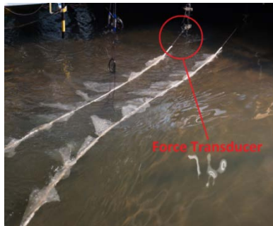
Figure 8-10: Impression of Saccharina modelled seaweed in the basin, where the load on the line is measured.
