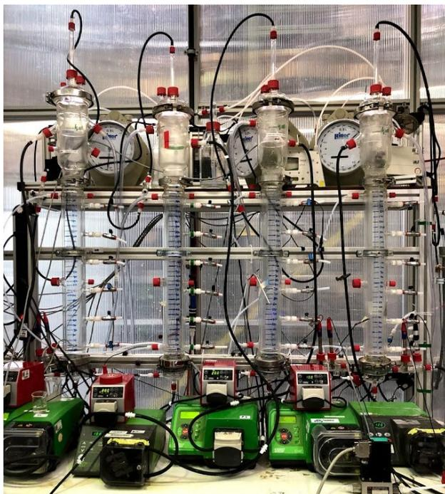
Figure 1 Lab-scale UASB reactors
