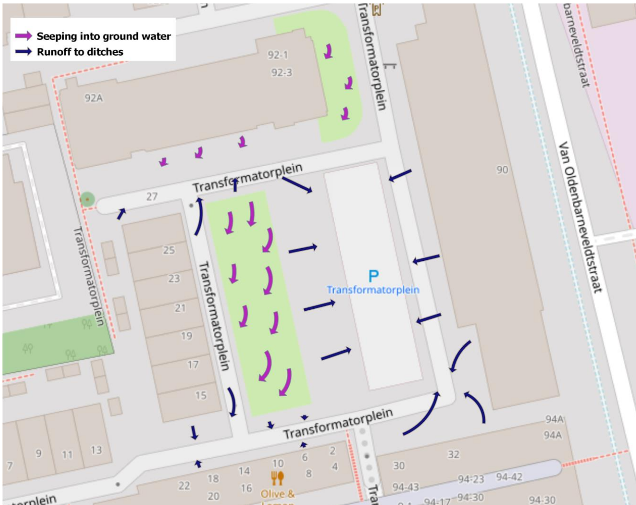
Figure 20 - A visualisation of precipitation both seeping into groundwater, which mainly occurs on the vegetated areas, and the rainwater running off towards ditches and thus into the sewage systems. The estimation is based on the slight slope present on the square's surface, the surface type (vegetated or not-vegetated) and the presence of ditches.
