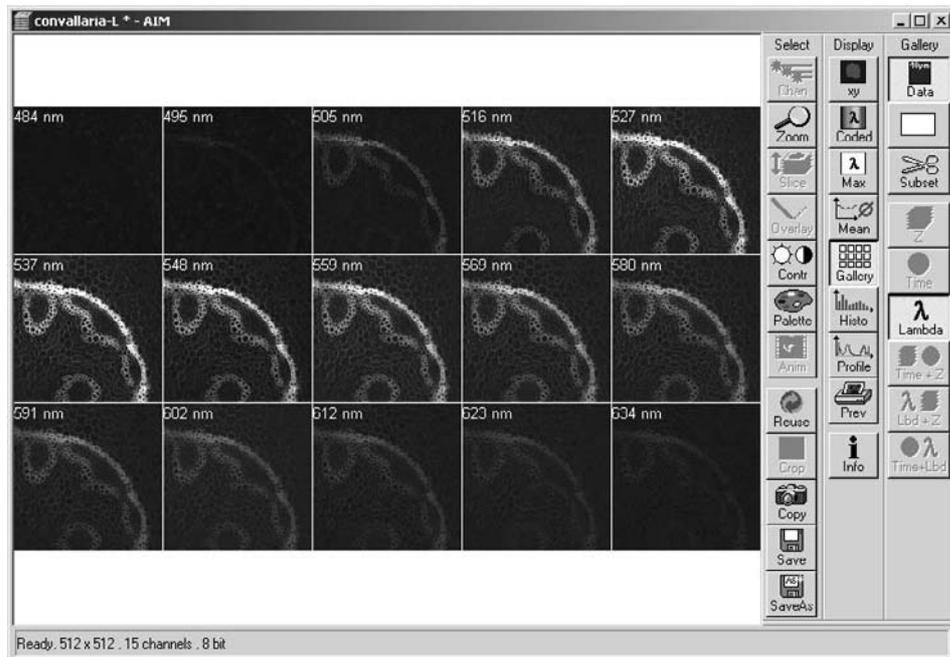
**Fig. 5-64** Image Display window with a Lambda Stack
