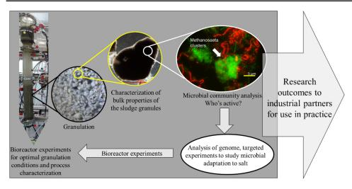
Figure 2: Research that made anaerobic granular sludge technology work for waters with high salinity.
