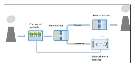
Figure 4: Technology train developed with and tested for Dow Benelux, to make cooling tower wastewater reusable.
