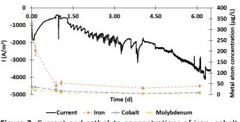
**Figure 2.** Current and catholyte concentrations of iron, cobalt and molybdenum during startup of an abiotic CO<sub>2</sub> fed reactor.
