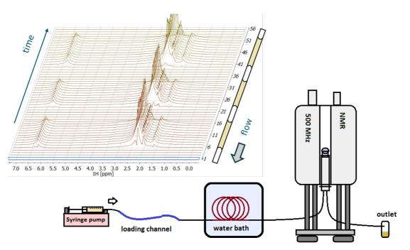
**Figure 1**, *Top*) NMR spectra collected over allow for a composition analysis of the reaction mixture. *Bottom*) the set-up: a slug flow of reactants is prepared in the loading channel and pushed through reactor and the NMR for in-line detection.
