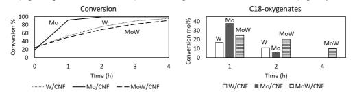
Figure 2. Stearic acid conversion over Mo/CNF, W/CNF and MoW/CNF (250 mg catalyst, 2 g stearic acid, 50 mL solvent, 30 bar  $H_2$ , T = 350 °C).
