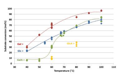
Reactions were carried out in a continuous flow reactor over a Au-catalyst bed. Each carbohydrate was evaluated over a temperature range between 40 and 100 °C. Conversion as a function of temperature is shown in Fig. 2.
