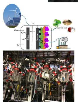
**Figure 1.** Schematic (top) and lab (bottom) setup of the microbial electrosynthesis system.
