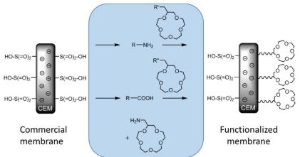
**Figure 3**. Possible membrane modification schemes to obtain a one-side, crown-ether-functionalized membrane. R' = OH/COOH,  $R'' = OH/NH_2$ .
