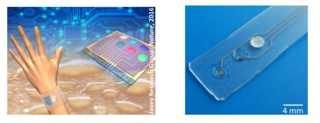
**Figure 1.** (Left) Schematic illustrations of a multiplexed perspiration analysis, showing a wearable sensor on a subject's wrist and a detail of the sensor lay-out containing several active sensors spots (source: Javey and co-workers, Nature, **2016**, *529*, 509–514), (right) Flexible screen-printed ion-selective sensor (courtesy: Holst Centre).
