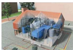
Wastewater treatment installation (Waterschoon) for black and grey water in Sneek.
