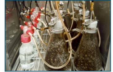
Gas evolution tests (CO 2 or CH 4 )
