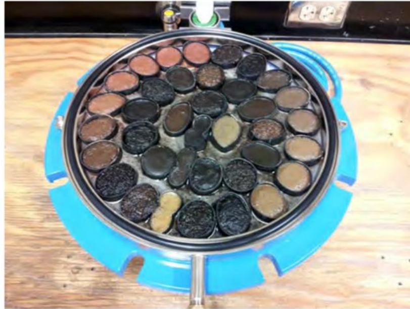
Figure 3C2a-2.—Pressure-membrane extraction at 1500-kPa for <2-mm samples.
