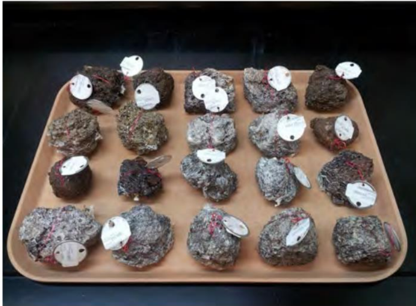
Figure 3B1b-1.—A round stock tag with sample identification number is prepared. The cut copper wire is looped around the clod.
