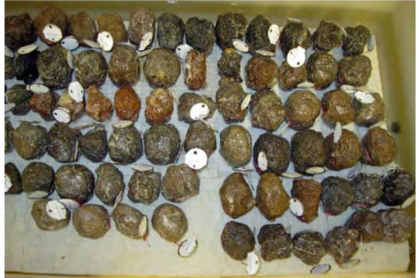
Figure 3B1b-2.—After a flat surface on the clod is cut with a diamond saw, the clod is placed on a tension table, maintained at 5-cm tension.
