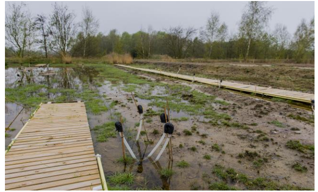
Test site for the newly developed submerged tubular system to generate plant electricity in Brabant. (Photo: Wild Frontiers)
