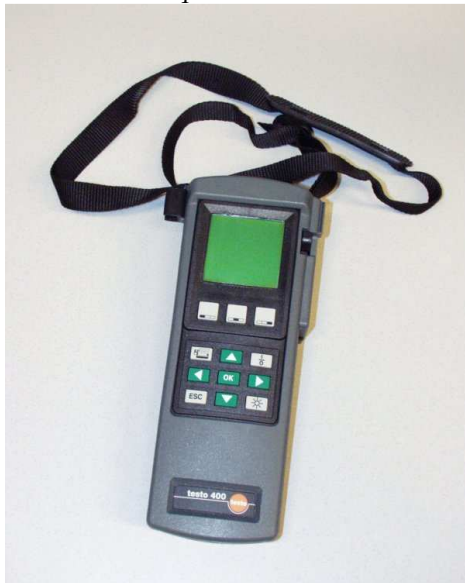
Fig. 10, testo400 handheld datalogger.
