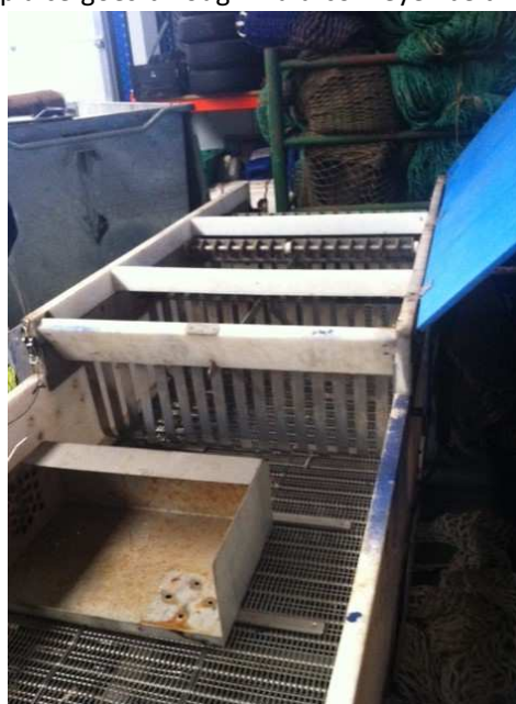
Figure 10. The electrical stunning machine that is used by Ekofish Group.
