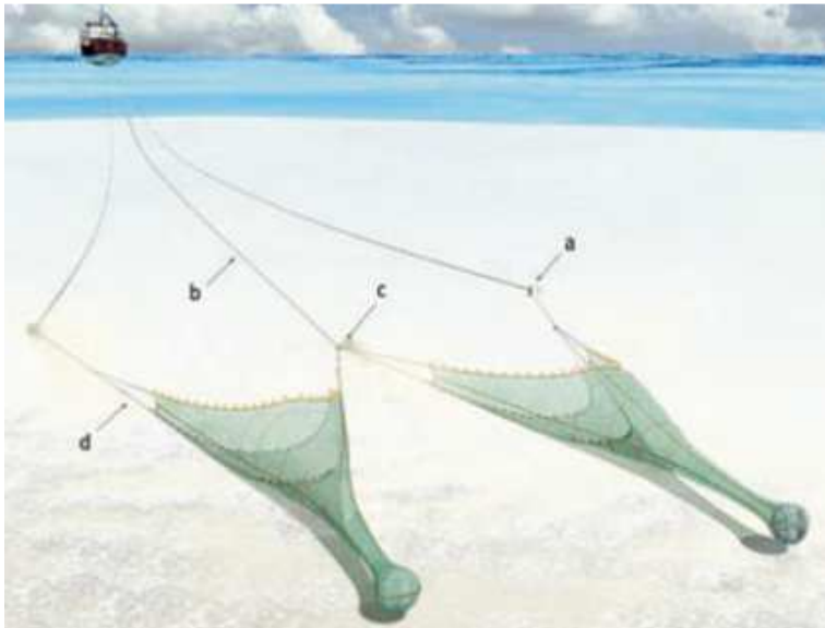
Figure 7. Twinrig; a = trawl boards, b = cable to the centre weighting block, c = centre weighting block, d = sweeps ( www.schmidtzeervis.nl , 7-4-2014).
