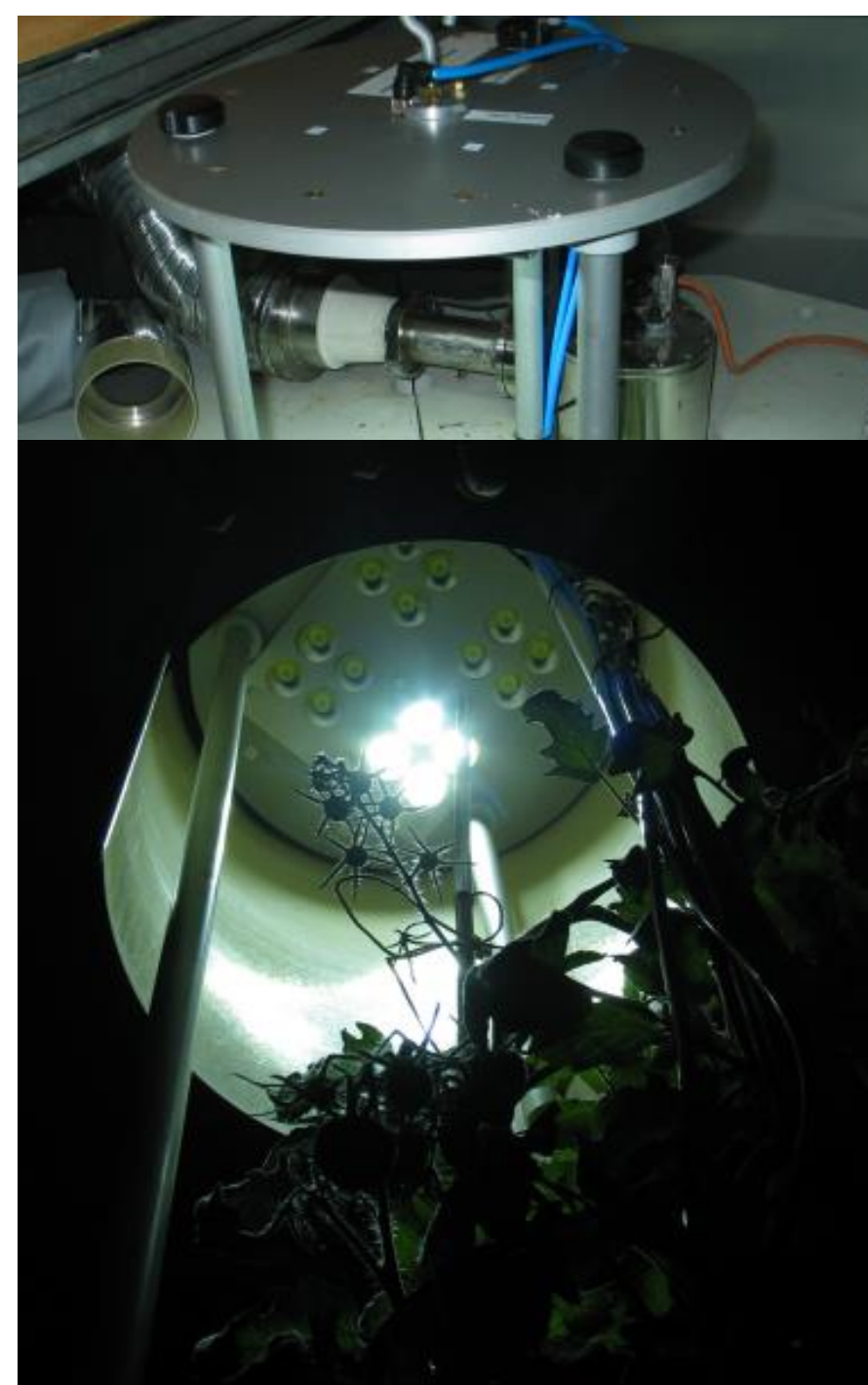
Figure 2. upper- cooling of LED module, lower - LED module
