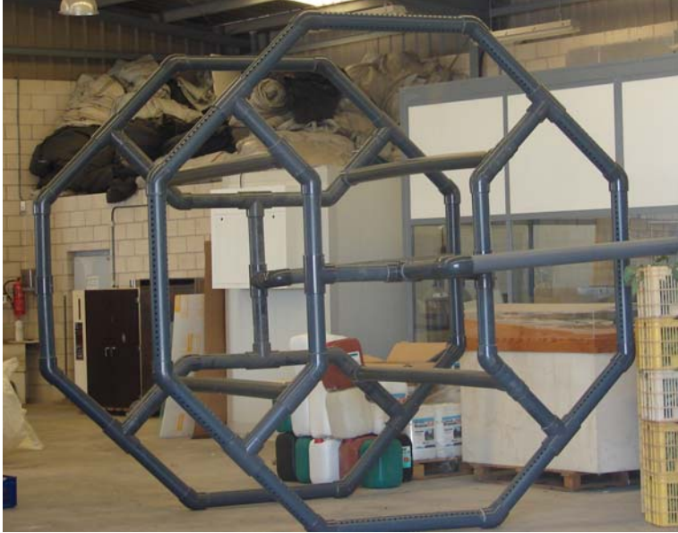
Fig. 33 Double diffuser finally constructed before final implementation in the silo
