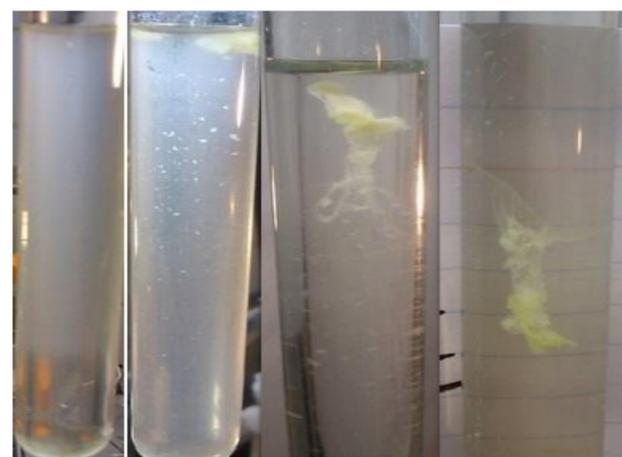
Figure 1: Formation of flock over time, algae exposed to 0.5 ml/l dispersant (Corexit 9500)
