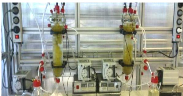
**Up-flow anaerobic filters with continuous production of MCFAs**
