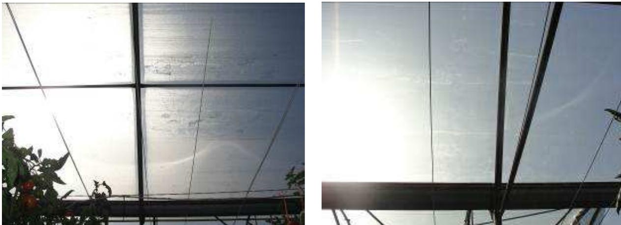
Figure 4.11. Left, control film showing condensation in the morning, and right, NIR\_film, without condensation.
