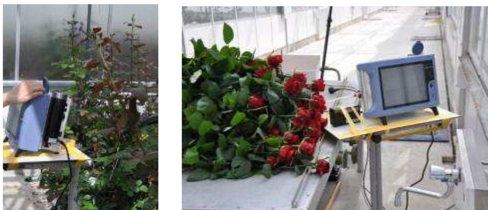
Figure 2.7. FAIMS measurements in the test greenhouse (right) and outside it (left) for scent background of harvested flowers.
