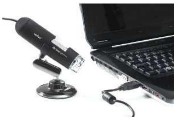
Figure 2.8. A hand-held digital microscope.
