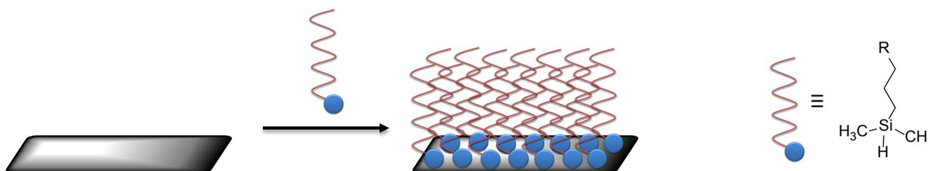
**Figure 1.** Schematic representation for the immobilization of hydrosilanes on a solid substrate.
