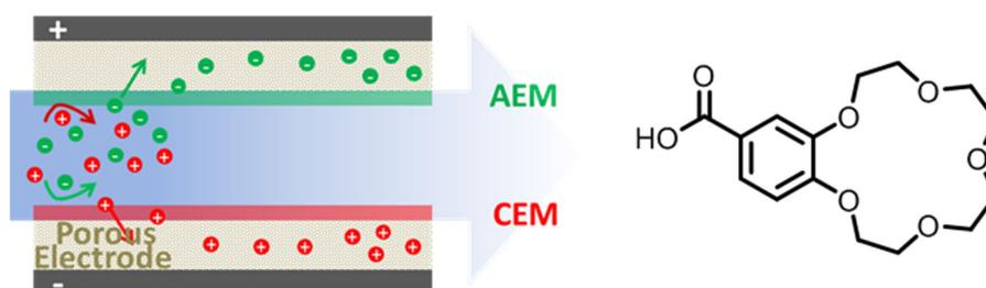
**Figure 1.** Left: Schematic representation of capacitive deionization with anion and cation-exchange membranes (AEM and CEM, respectively). Right: The structure of an  $\text{Na}^+$ -selective molecule that will be used to functionalize the porous electrodes.
