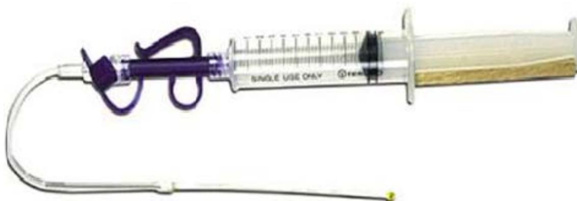
Rhizon Soil Moisture Sampler for extracting nutrient solution from growing medium.
