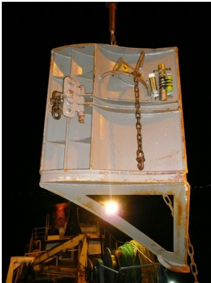
Figure 7.4.7. Full-scale prototype of the Jumper Door developed by Morgère and Ifremer (image courtesy of Benoit Vincent - Ifremer).
