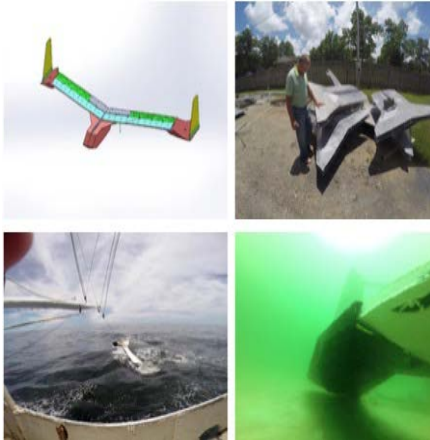
Figure 7.4.14. Wing Trawling System used for tropic shrimp trawling in the Gulf of Mexico ( images courtesy of Philip Walsh – Memorial University )
