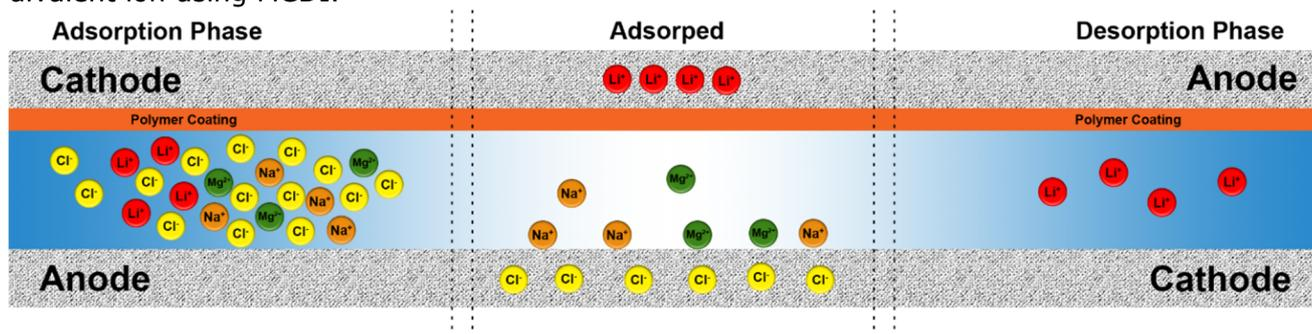
**Figure 2.** Conceptual representation of the proposed MCDI setup. The cathode is coated with a polymer layer that selectively adsorbs Li<sup>+</sup> ions. Once the electrode is saturated with Li<sup>+</sup>, the rest of the ions are flushed out of the stream, followed by desorption of Li<sup>+</sup> ions by reversing the electrical field, ideally generating a Li<sup>+</sup> rich stream.
