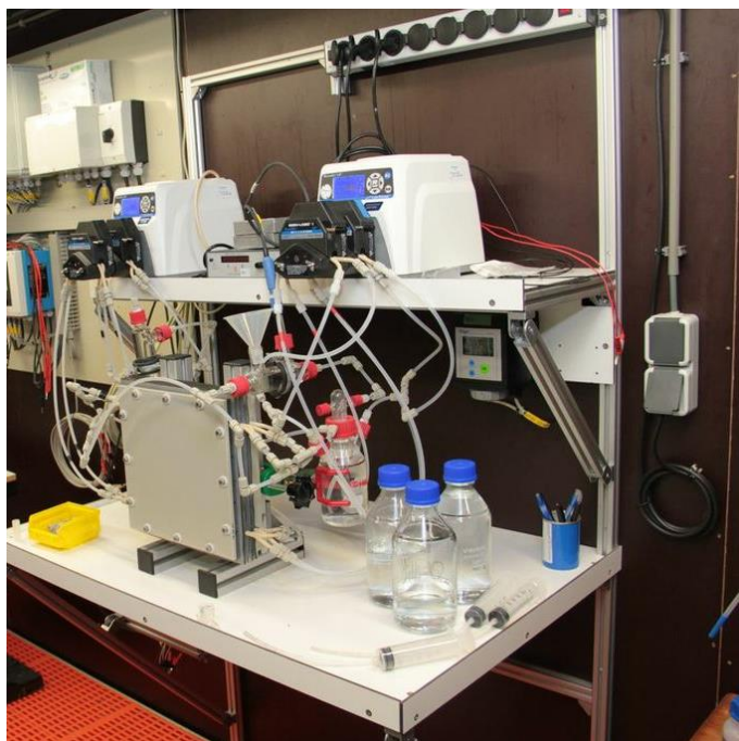
Fig. 2 The first pilot study on the recovery of energy and nutrients from urine at the Wetterskip Fryslân.
