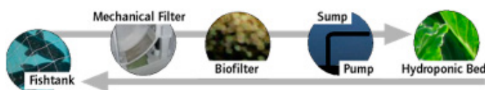
Figure 2.2. Basic aquaponic system layout.
