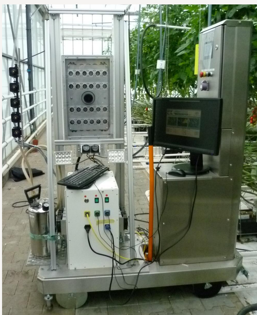
Camera system equipped with stereo-vision and CF-technology
