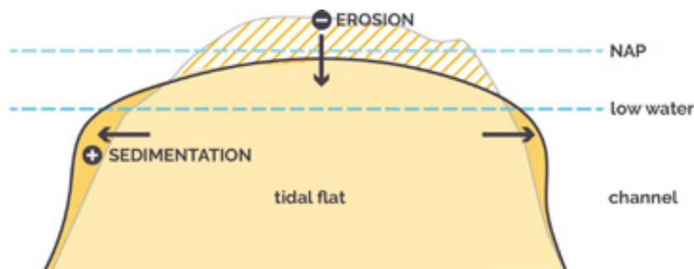
Fig. 34. The main problem caused by the OSB: erosion of the tidal flats, due to decreased flow velocity in the channels, and decreased tidal volumes. Adapted from: (Zanten & Adriaanse, 2008).
