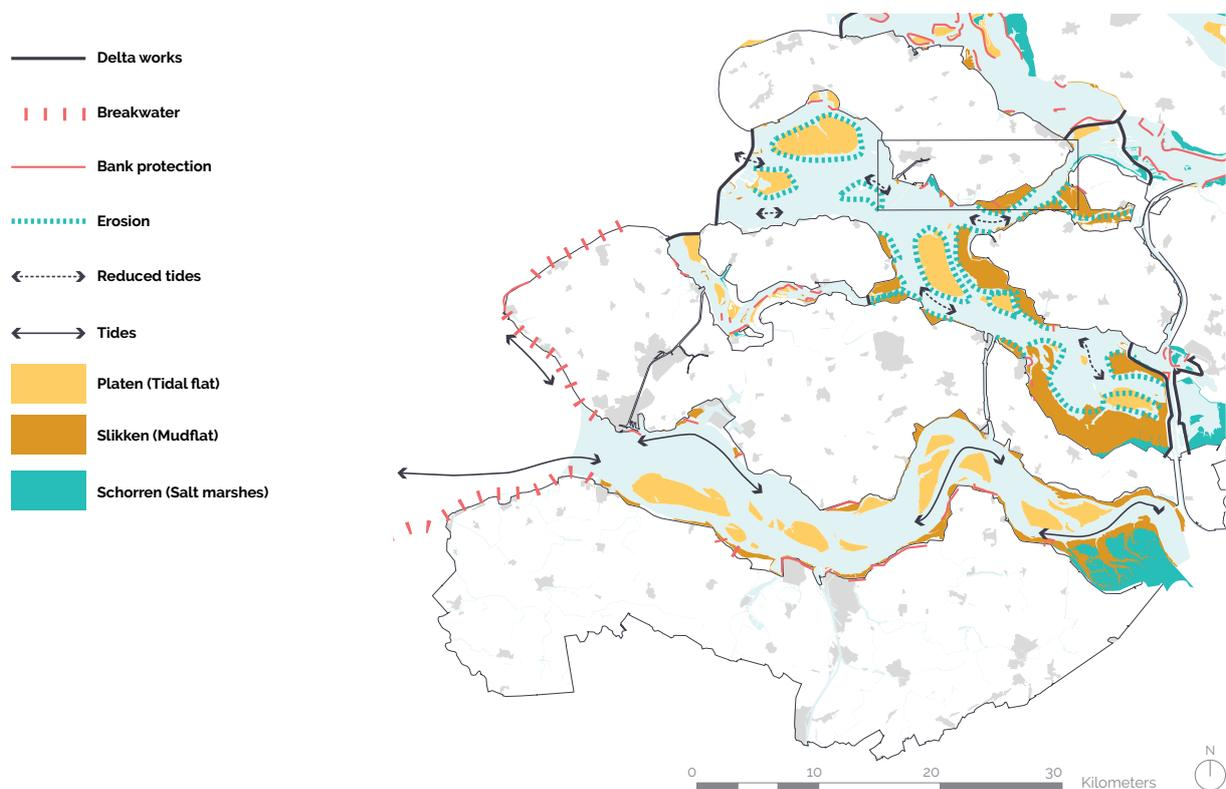
Fig. 33. Erosion and tidal changes in the morphological system caused by the Delta Works. Adapted from Meyer, Bregt, Dammers, & Edelenbos, (2015); Provincie Zeeland (2019).
