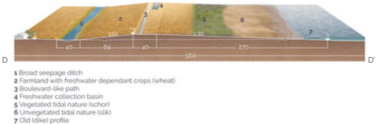
Fig. 79. Overview of the new tidal super dike and the different elements, dimensions in meters (m), heights in relation to NAP.
