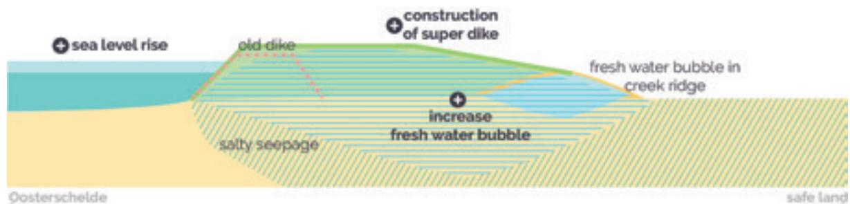
Fig. 50. Developed intervention: super dike situated on the edge of a freshwater bubble and salt groundwater.
