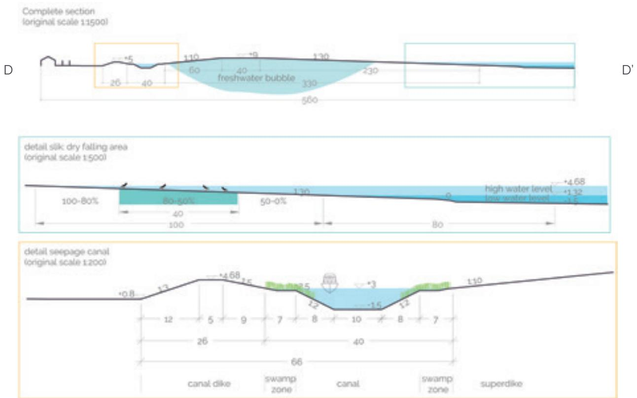
Fig. 66. The section of the super dike illustrates the freshwater bubble, the tidal nature, and the seepage canal, dimensions in m, heights in relation to NAP.
