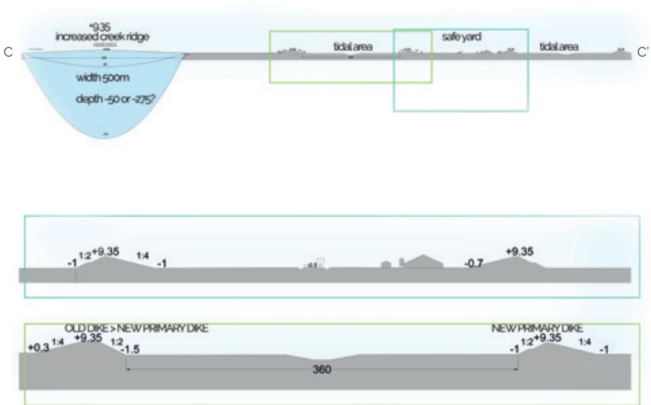
Fig. 58. Sections illustrating the new freshwater bubble, the new tidal nature, and the safe yard. Dimensions in m, heights relative to NAP.
