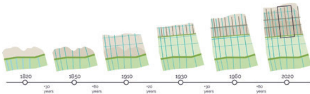
Fig. 43. Enhancing sedimentation using the salt marsh works system ('kwelderwerken'), as found in the North of the Netherlands. Adapted from Kadaster (2019).
