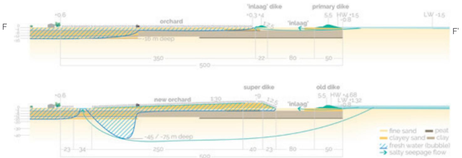
Fig. 83. Section of the existing situation (top) and the new agricultural super dike (below), dimensions in meters (m), heights in relation to NAP. HW: high water level, LW: low water level. Adapted from (TNO, n.d.). Location of section indicated in Figure 73.
