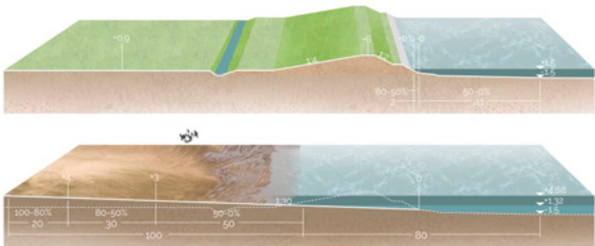
Fig. 80. The old profile (top) and the new unvegetated tidal nature at the start of the super dike (below), dimensions in meters (m), heights in relation to NAP.
