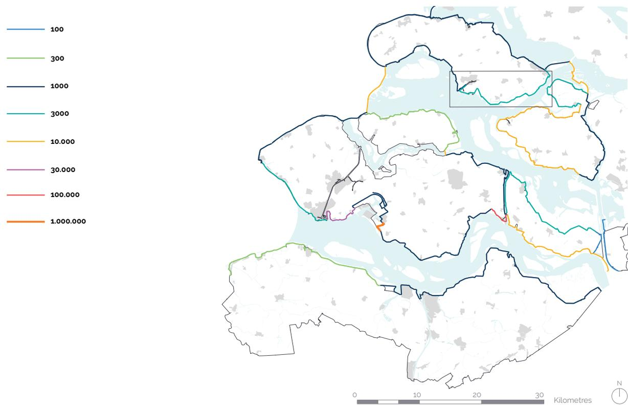
Fig. 31. Protection standards (lower limit). Adapted from Slootjes & van der Most (2016).
