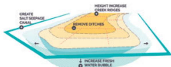
Fig. 56. Designing the creek ridge to enlarging the freshwater bubble.
