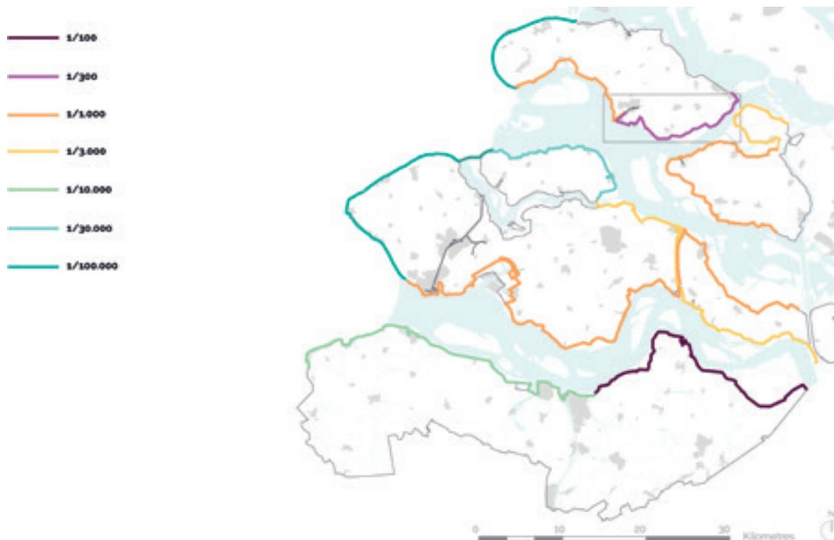
Fig. 32. Flood chances per dike trajectory, after completion of projects in 2020. Adapted from Slootjes & van der Most (2016).
