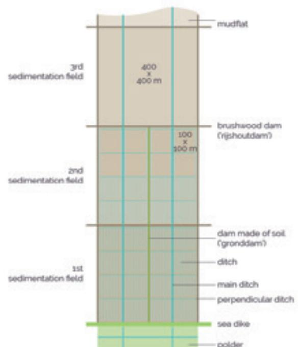
Fig. 45. Detailed principle of salt marsh works ('kwelderwerken'), m = meter. Adapted from van Duin et al. (2016).
