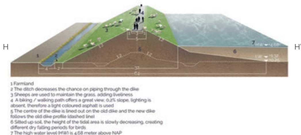
Fig. 87. Section of the upgraded secondary dike. Dimensions in m, heights relative to NAP, HW: high water level, LW: low water level. Location of section indicated in Figure 75.
