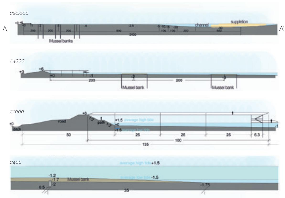
Fig. 48. The sections show the interventions: the elevated recreation element, the mussel banks, and the suppletion. Dimensions in m, heights relative to NAP.
