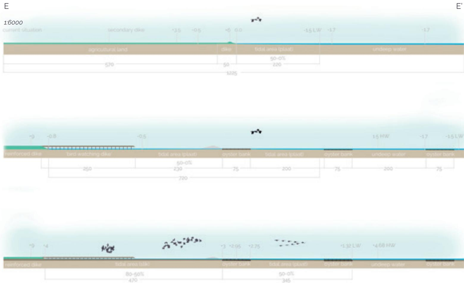
Fig. 70. A - Transition from the existing situation (top), the intervention (middle), and the 'final' situation (down). By silt suppletions, the tidal area silts up heigher and oyster banks grow with SLR. Dimensions in m, heights in relation to NAP. HW: high water level, LW: low water level.
