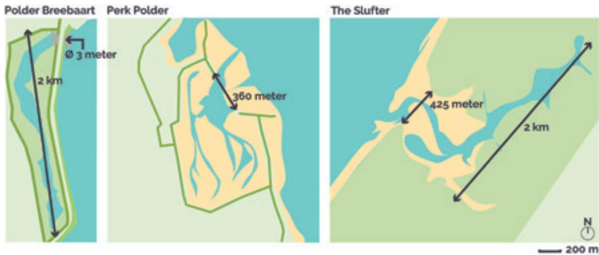
Fig. 51. Studied inlet widths for the development of a new tidal nature area landward. Km: kilometre.
