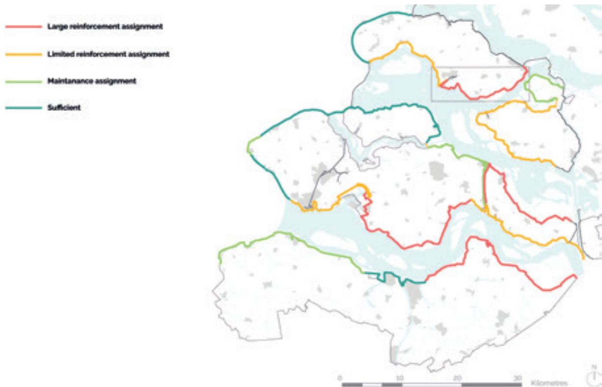
Fig. 6. Reinforcement assignment for the south-western delta on basis of the new norms. Adapted from Slabbers (2014).
