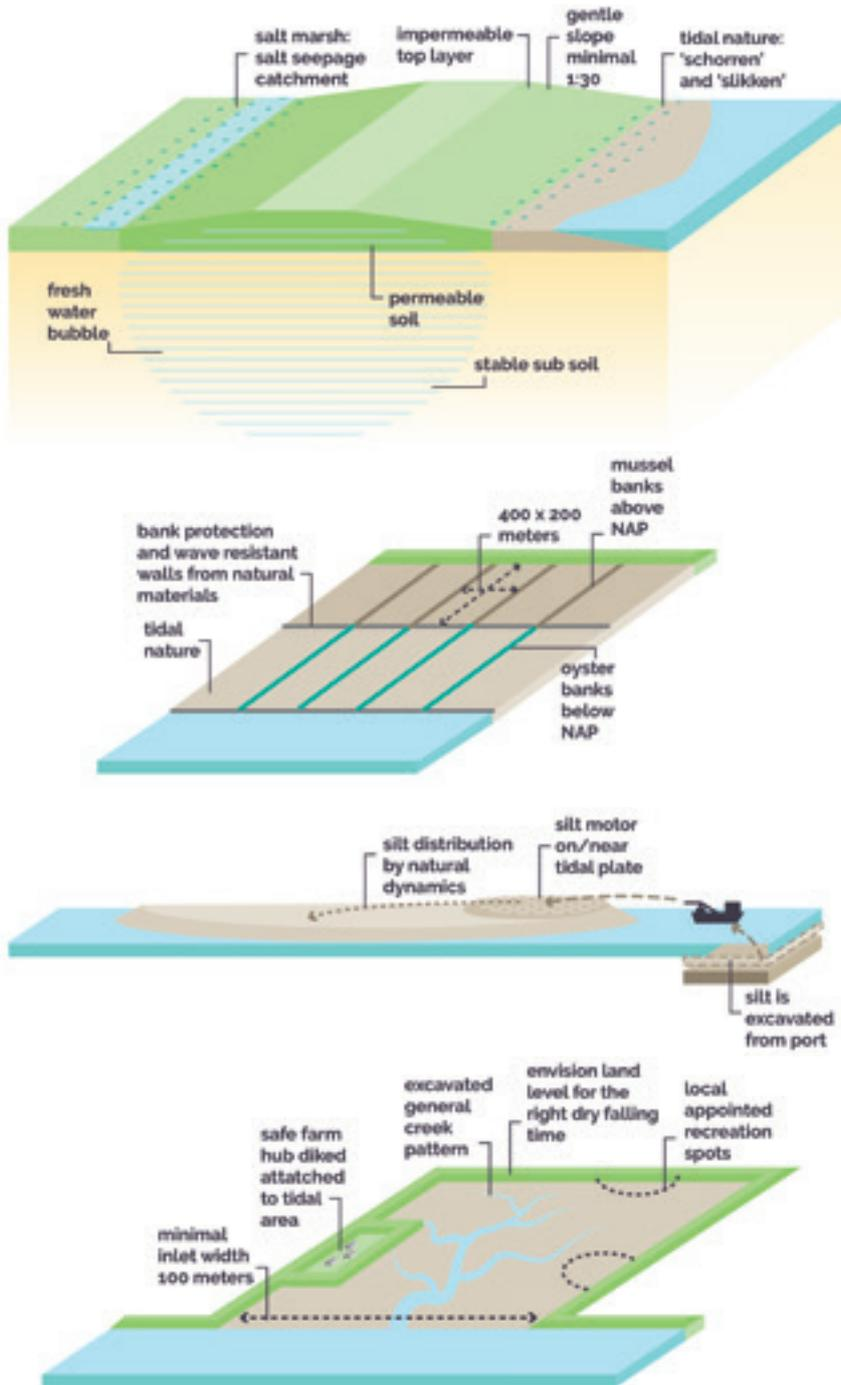
Fig. 64. The principles based on the selected interventions, from top to down: super dike, tidal grid, silt motor, and new tidal nature landward.
