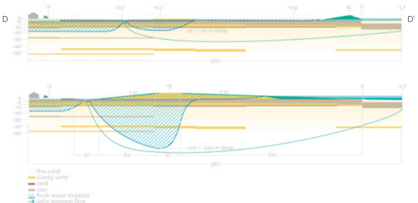
Fig. 78. Section of the existing situation (top) and the new tidal super dike (below), dimensions in meters (m), heights in relation to NAP. Adapted from (TNO, n.d.).
