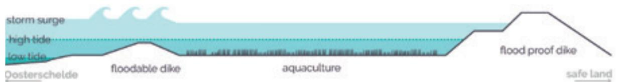
Fig. 49. Two types of double dikes resulting in a different type of land use. Adapted from Dieker & Veendorp (2020).
