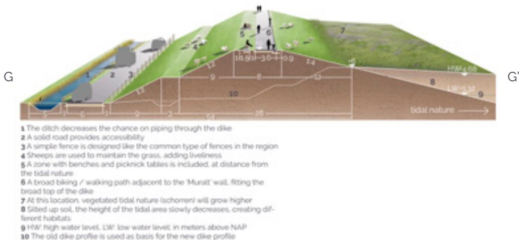
Fig. 86. Section showing the primary dike. Dimensions in m, heights relative to NAP, HW: high water level, LW: low water level. Location of section indicated in Figure 75.
