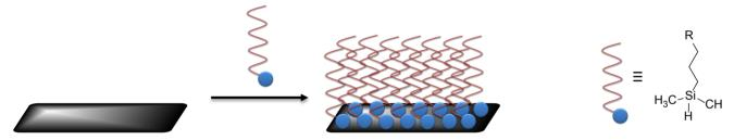
Figure 1. Schematic representation for the immobilization of hydrosilanes on a solid substrate.
