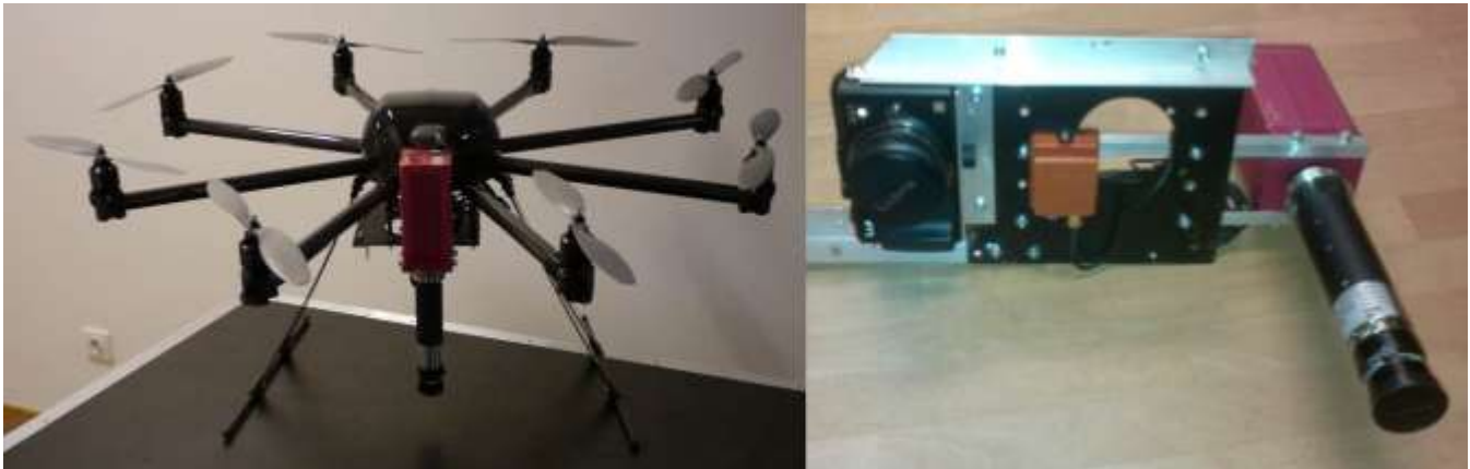
Figures 1a and 1b. Aerialtronics Altura AT8 octocopter and the hyperspectral mapping system. The system consists of a Panasonic Lumix GX1 camera, XSens MTi-G-700 INS, and a pushbroom spectrometer.
