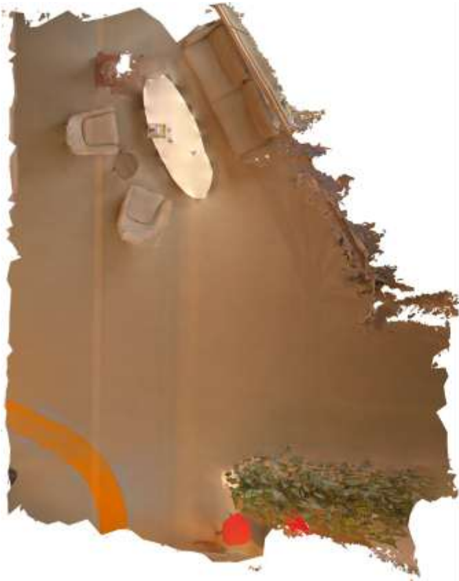
Figures 3a and 3b. An orthomosaic and a DSM created from the Panasonic GX1 images using photogrammetric methods (Agisoft PhotoScan Pro).
