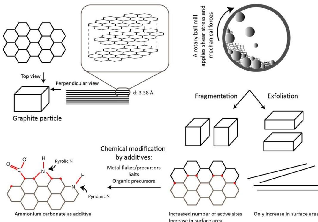
**Figure 1.** Illustration of the graphite structure and its physiochemical modification by a rotary ball mill
