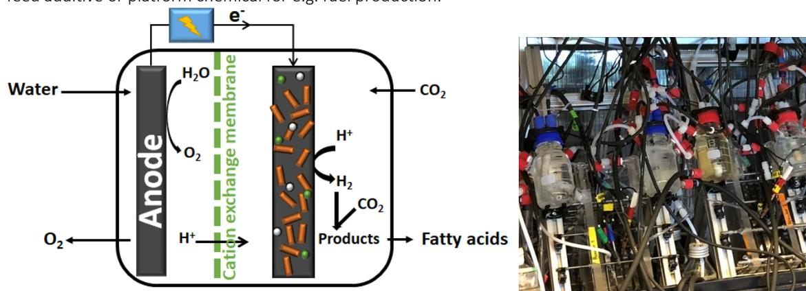
**Figure 3.** Schematic (left) and actual (right) setup of bioelectrochemical chain elongation systems.
