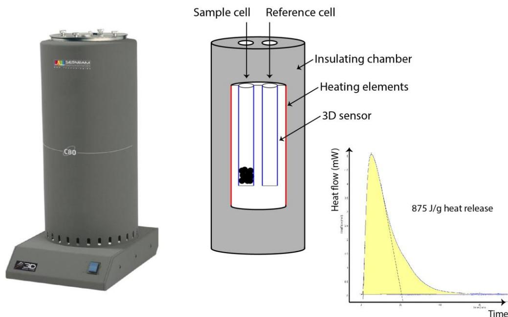
**Figure 1.** A photo of C80 calorimeter (left), illustration of its components (middle), and a graph showing heat release during CO<sub>2</sub> capture from air upon exposure to supported K<sub>2</sub>CO<sub>3</sub> based sorbent (right)
