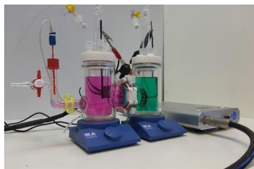
**Figure 1.** H-cell used for preparative electrolysis.
