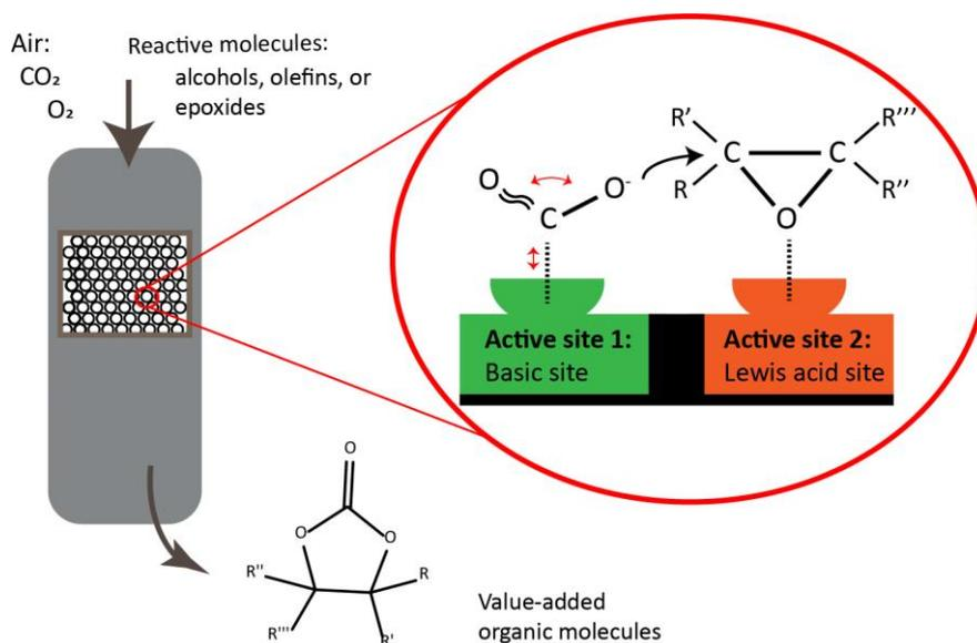
**Figure 1.** Rational design of bifunctional solid catalysts to convert CO<sub>2</sub> to organic molecules
