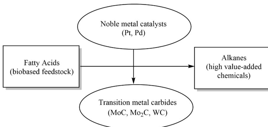
*Figure 6: Scheme for biomass conversion. The horizontal flow shows the conversion of fatty acids into alkanes in the presence of a heterogeneous catalyst. The vertical flow indicates the substitution of noble metal catalysts with the transition metal carbide catalysts.*
