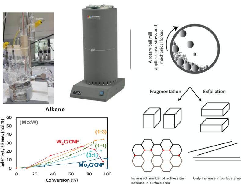
Some examples: electrochemical reactor for biobased conversions (top left), commissioning of a C80 calorimeter for operando heat measurement (top middle), modification of carbons by ball milling (right) and steering selectivity of Mo/W-carbide catalysts for deoxygenation of stearic acid (bottom left)
