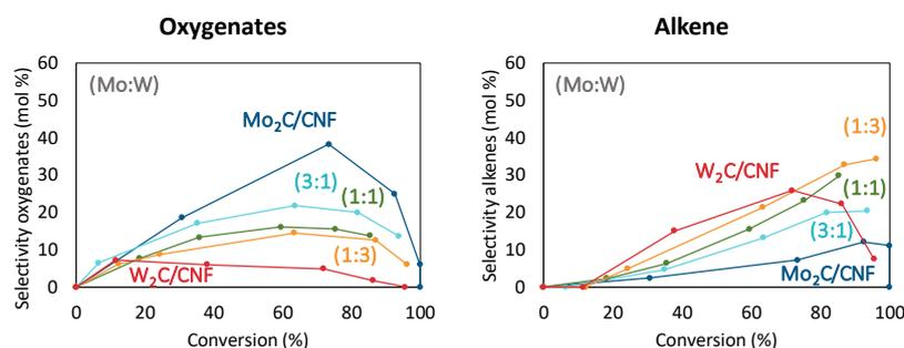
Figure 2. Conversion vs selective of oxygenates and alkenes of mixed metal carbides synthesized (250 mg catalyst, 2 g stearic acid, 50 mL solvent, 30 bar H<sub>2</sub>, 350 °C).
