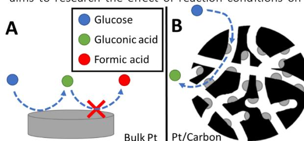
Figure 1. A) the system setup under which the effect of reaction conditions will be studied for the selective conversion of glucose and B) a representation for the model for high surface area electrodes (Pt/CNF), that will be used to study the effect of design parameters on the electrocatalytic oxidation of glucose
