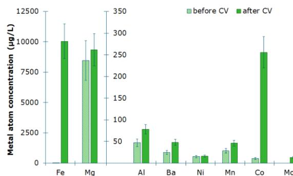
**Figure 4.** Metal concentrations in the reactor liquid before and after cyclic voltammetry (CV).
