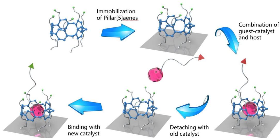
**Figure 1.** Schematic illustration of immobilization pillararenes on support and regeneration of deactivated catalysts with stimulations.
