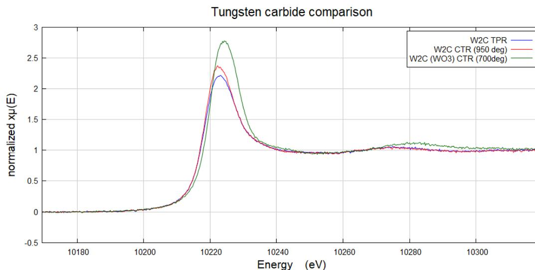
**Figure 1:** XANES measurement of three different samples:  $\text{W}_2\text{C}$  synthesized by carbothermal reduction (CTR) at 950°C (red),  $\text{WO}_3$  created by incomplete CTR at 700°C (green);  $\text{W}_2\text{C}$  prepared by thermal programmed reduction (TPR) at 700°C under 80/20  $\text{H}_2/\text{CH}_4$  flow (blue).
