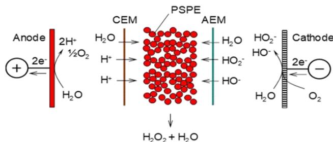
**Figure 2.** Cell design for the electrochemical production and in-situ concentration of  $\text{H}_2\text{O}_2$ .
