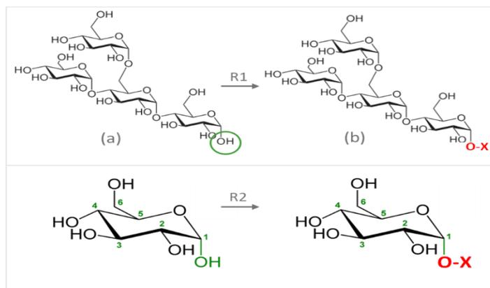
Figure 1: Selective pre-treatment (R1; i.e. reaction 1) of a starch molecule (a) that results in blocking of the terminal carbon (b). The same reaction (R2) has been previously shown for the glucose molecule.
